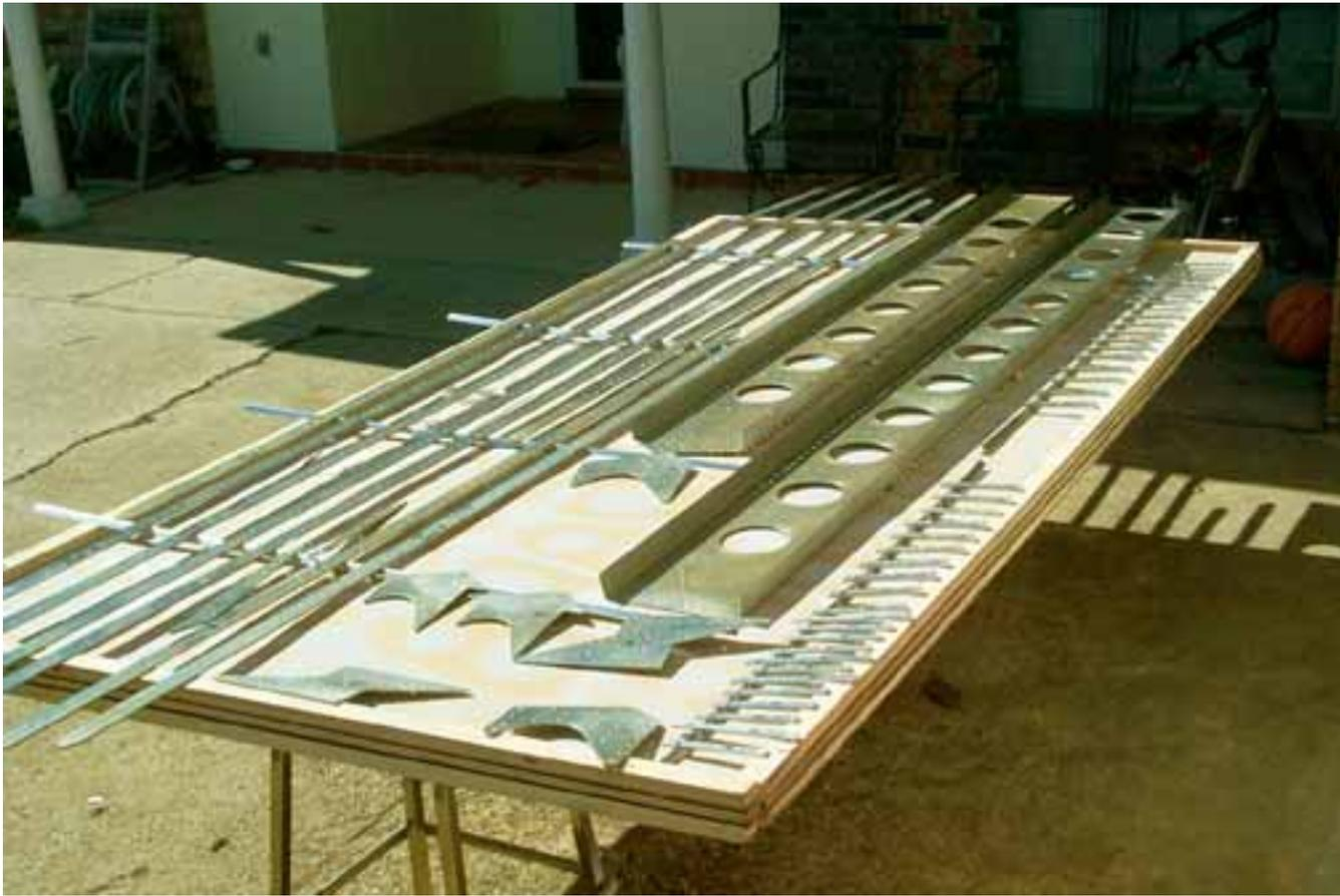
The parts were then allowed to air dry completely overnight. It is important to not rush this drying process. If your parts are still wet when you prime them, you will trap moisture between the primer and the part. Also, do not wipe the part dry. Just let it air dry. The parts will take on a kind of yellowish hue after the Alodine process. This is the protective coating, do not scratch it or rub it off.
