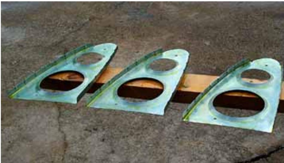
The Alodine is allowed to soak for about 5 to 10 minutes (do not let it dry, re-spray if necessary to keep wet) and then was rinsed off thoroughly with clean water. **Do not handle the parts with your bare hands.** You may get oil from your hands on the parts. When done correctly, the aluminum will have a golden, yellowish color to it.
