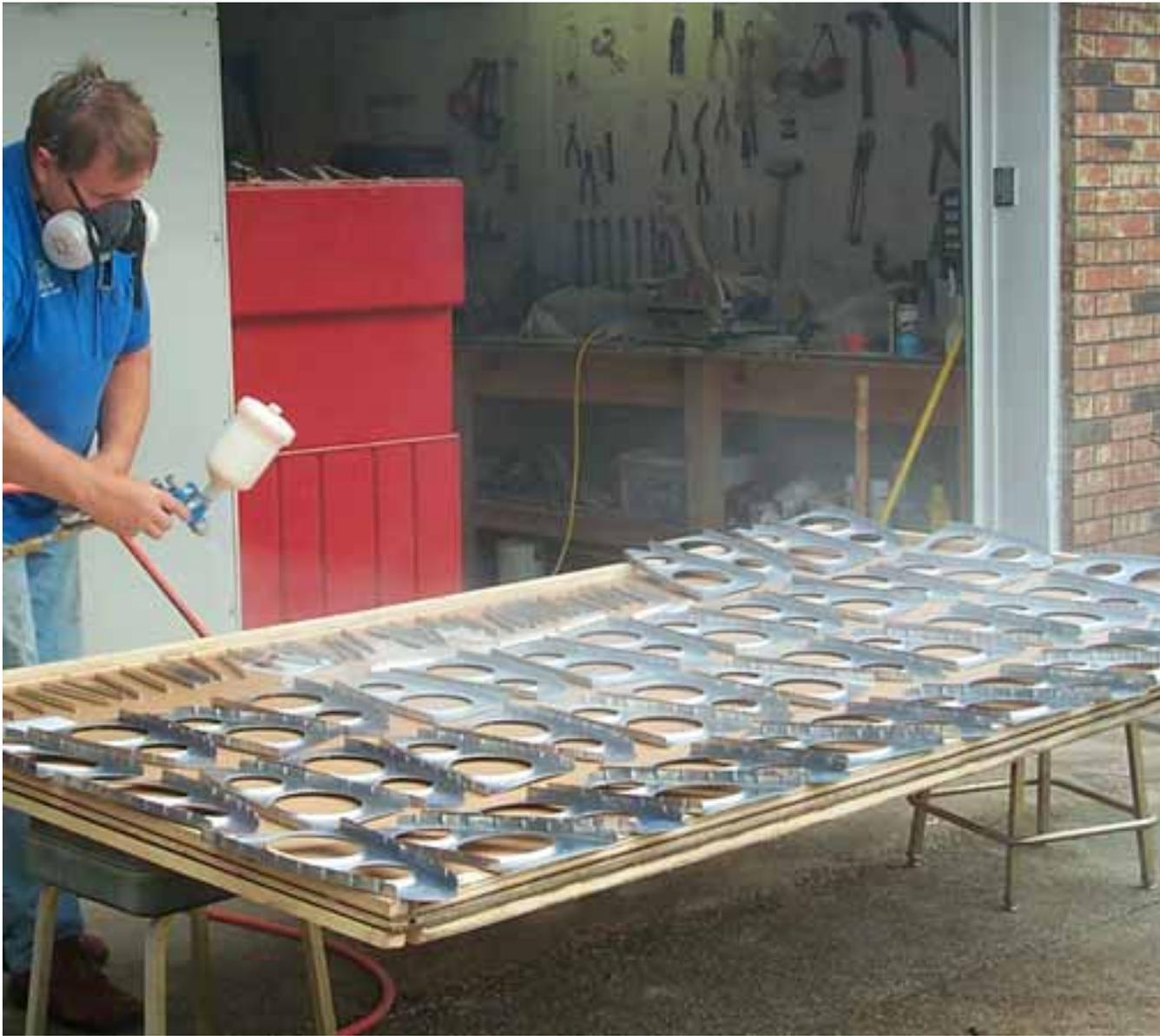
In the picture above I'm actually too far from the ribs that I'm priming. If done correctly, you won't have nearly all of the overspray I was creating in the above photo and less waste as well. During spraying, I concentrated on getting a good coat on the mating surfaces mostly. Any place where the parts will come together (stiffener to rib area, rib flanges, etc.) is more susceptible to corrosion than a part that is simply standing in mid air with nothing touching it.
