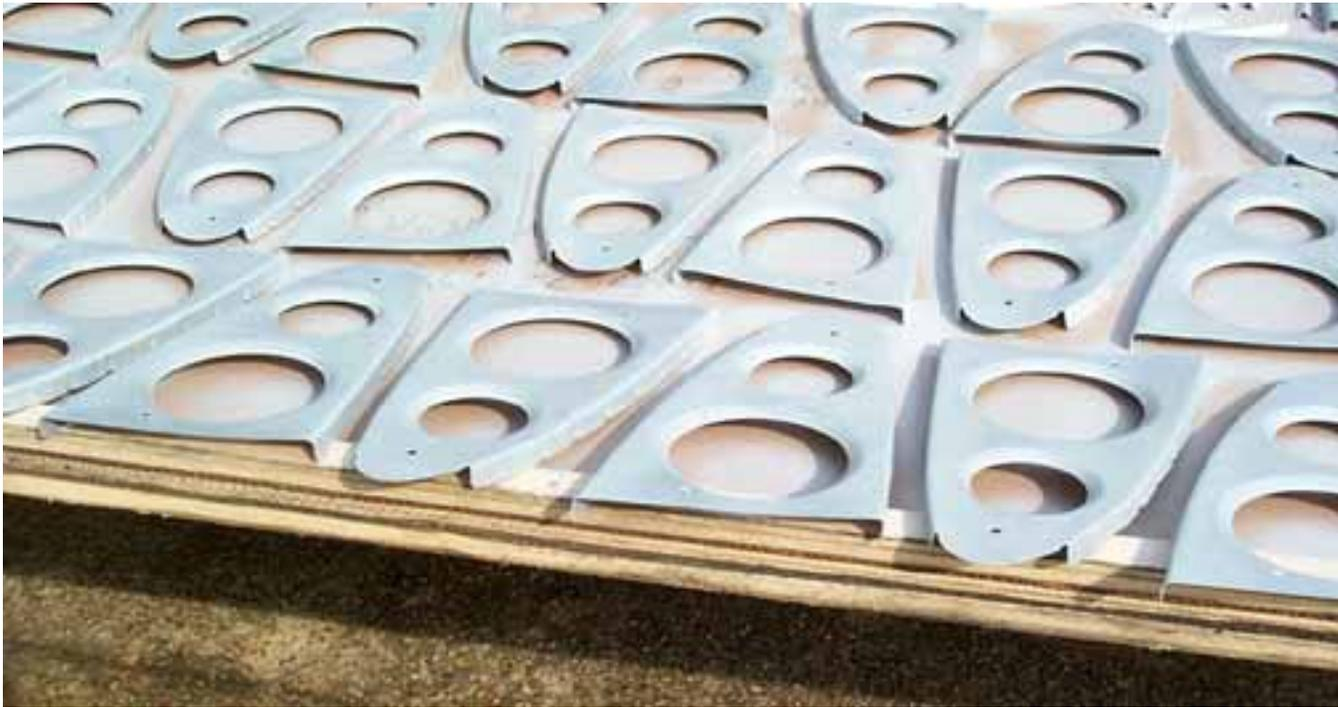
The stiffeners also received a coat of primer, mostly on the side that will touch the rib.
