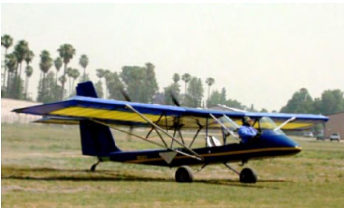
Look what showed up at the Low & Slow Fly-In! The king of low and slow...the twin-engined AirCam. The AirCam was developed by Phil Lockwood for the National Geographic Society's use in the Congo Basin. Its twin Rotax 912 engines gives it a landing roll of about 300 feet and a take-off roll of under 200 feet. The kit, less instruments, crating, shipping, and paint sells for about \$100,00.
